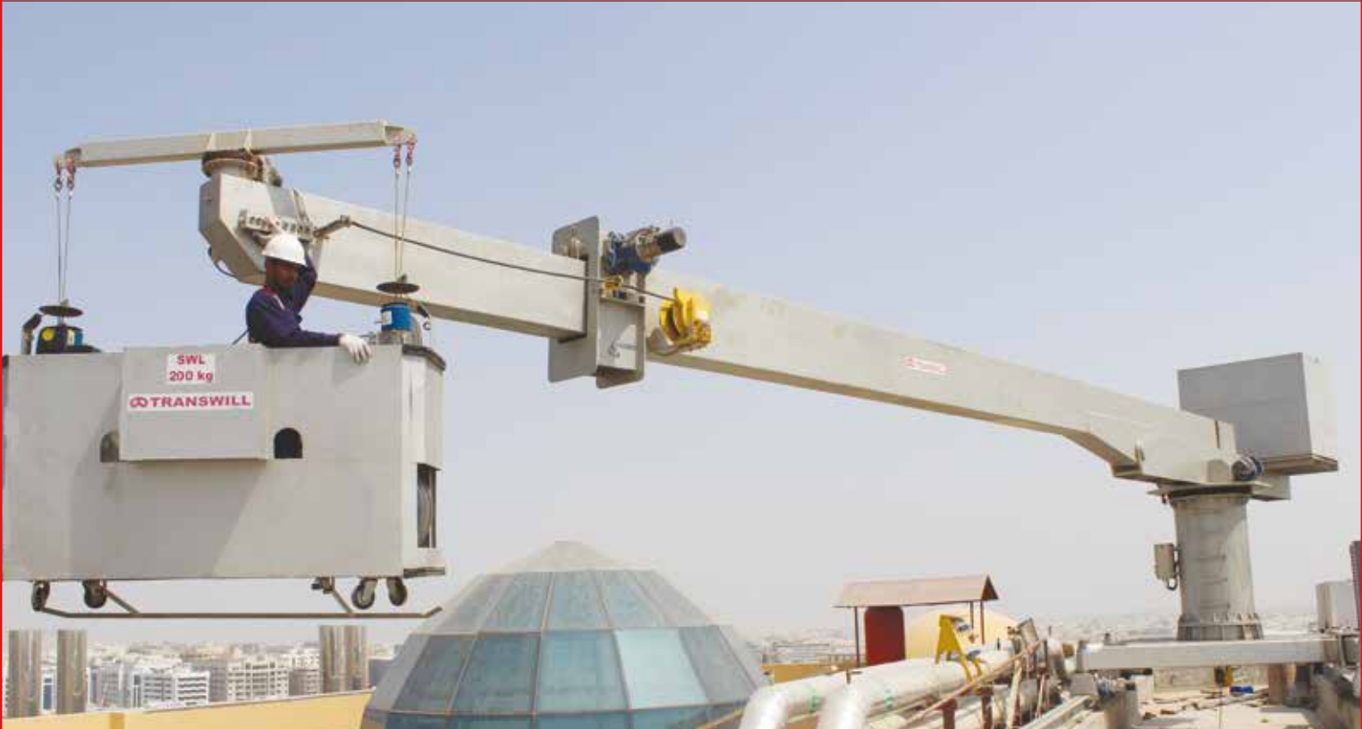
TWIN TRACK ROOF MACHINE (LONG REACH)
