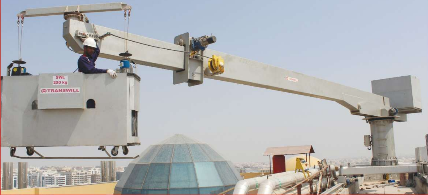
TWIN TRACK ROOF MACHINE (LONG REACH)
